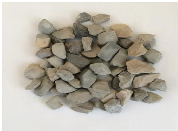
Fig 1. Simply crushed recycled coarse aggregate [10]
