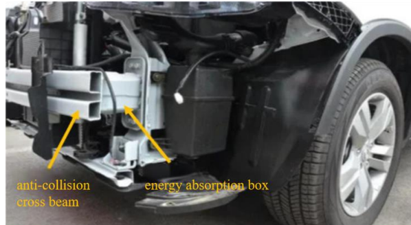
Figure 5. Automotive Anti-Crash Beam Structure[15]
